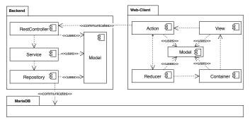
Fig. 1. Architecture of the system with the layers and the relationships between them
