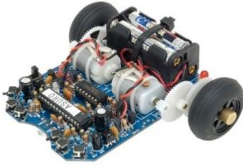
Figure 1. The ASURO robot with standard equipment
